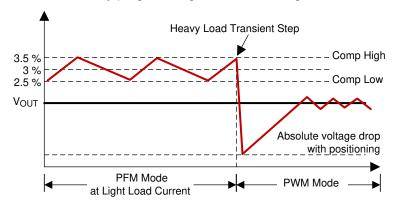
Figure 8-4. Power-Save Mode Thresholds and Dynamic Voltage Positioning
