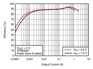
**Efficiency vs Output Current**
