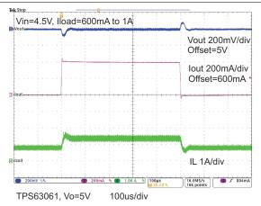
Figure 9-15. Load Transient Response
