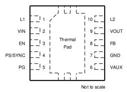
Figure 6-1. DSC Package 10 Pins (Top View)
