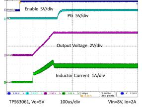
Figure 9-19. Startup After Enable
