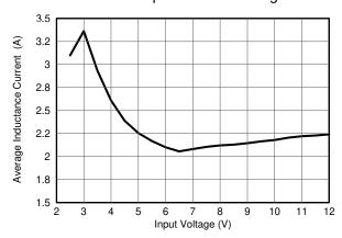
Figure 8-5. Average Inductance Current vs Input Voltage
