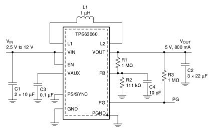
Figure 9-1. 5-V Adjustable Buck-Boost Converter Application
