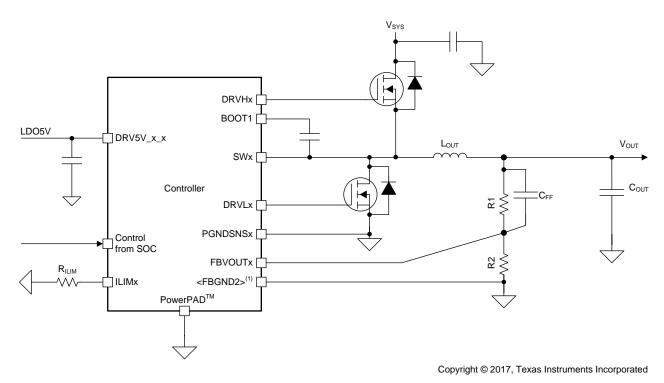
Figure 6-4. Controller Diagram With External Feedback Resistor
