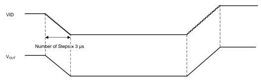
Figure 5-4. DVS Timing Diagram I (BUCKx\_DECAY = 0b)
