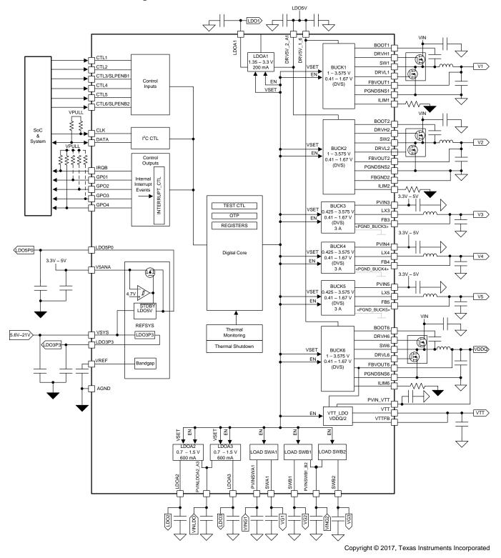
Figure 1-1. PMIC Functional Block Diagram
