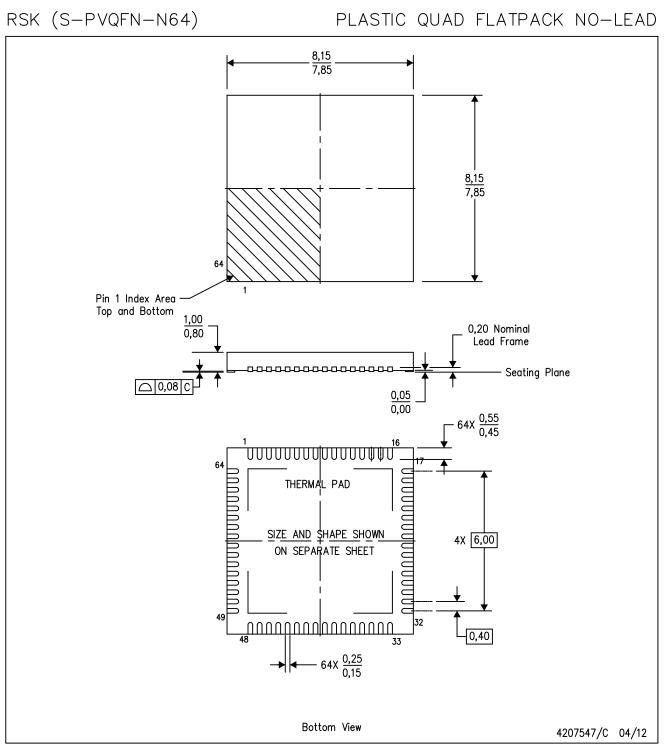
NOTES: All linear dimensions are in millimeters. Dimensioning and tolerancing per ASME Y14.5-1994. A.
