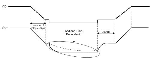
Figure 5-5. DVS Timing Diagram II (BUCKx\_DECAY = 0b)
