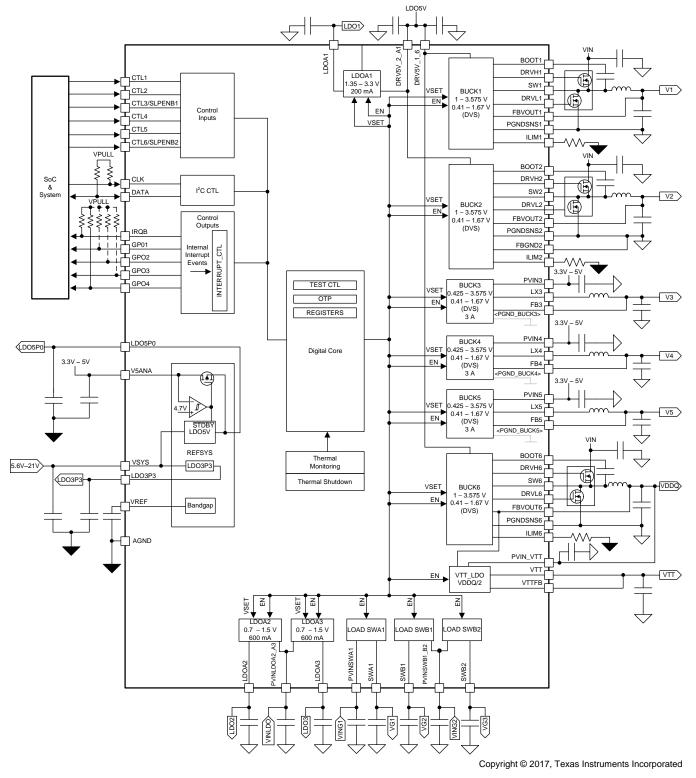
Figure 5-1. PMIC Functional Block Diagram
