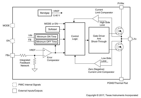
Figure 5-3. Converter Block Diagram
