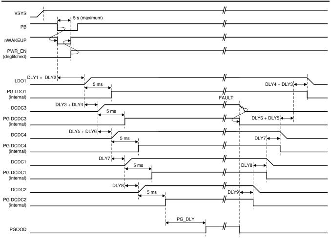
A. (1) Sequence shown for TPS65218D0 variant. For other TPS65218xx variants, refer to registers SEQ1-7 in Section 5.6.4 for factory programmed sequence order and timing.
