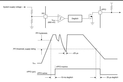
Figure 7-17. Power-Fail Comparator Simplified Circuit and Timing Diagram
