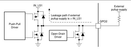
Figure 7-23. GPO2 as Open-Drain Output
