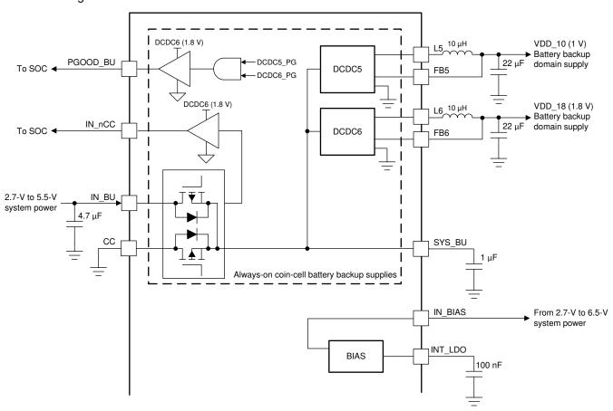
Figure 8-1. CC Input to Power Path
