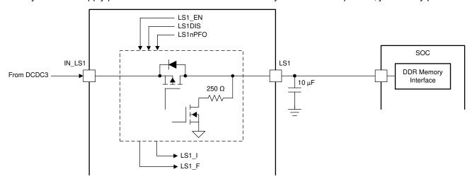
Figure 7-11. Typical Application of Load Switch 1
