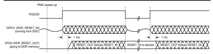
Figure 7-25. DDR3 Reset Timing Diagram
