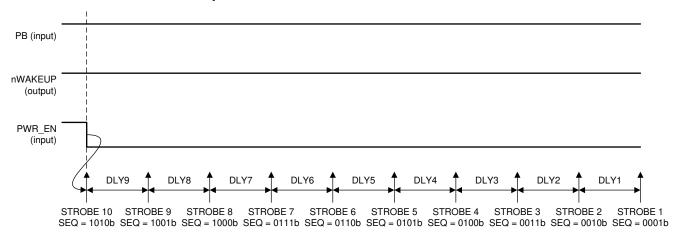
Figure 7-4. Power-Down Sequences to OFF State; PWR EN is Power-Down Event; FSEAL = 0b
