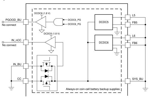
Figure 8-2. DCDC5 and DCDC6 Pins
