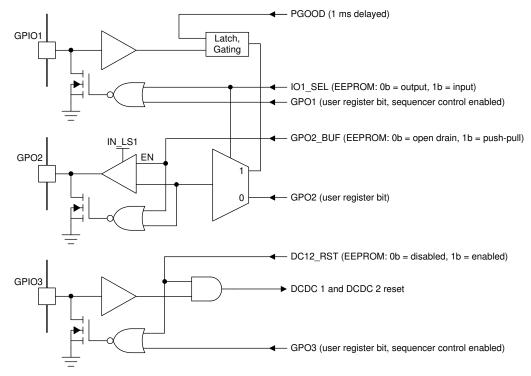
Figure 7-24. I/O Pin Logic
