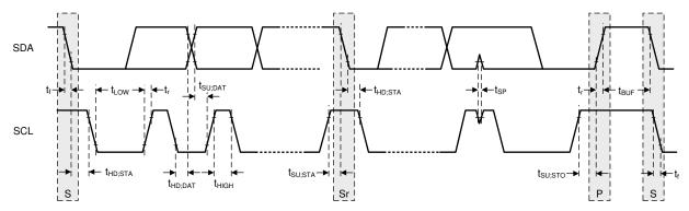
Figure 7-34. I<sup>2</sup>C Protocol and Transmission Timing I<sup>2</sup>C Data Transmission Timing
