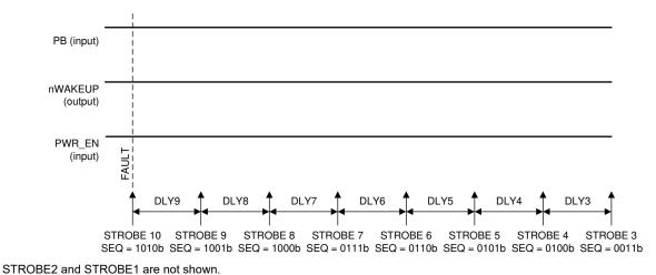
Figure 7-6. Power-Down Sequences to RECOVERY State; TSD or UV is Power-Down Event
