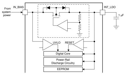
Figure 7-10. Internal LDO and UVLO Sensing
