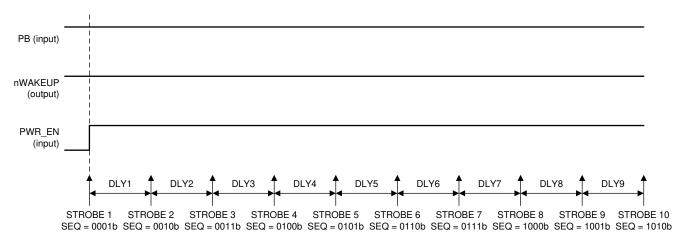
Figure 7-2. Power-Up Sequences from SUSPEND State; PWR\_EN is Power-Up Event
