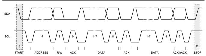
Figure 7-33. I<sup>2</sup>C Protocol and Transmission Timing I<sup>2</sup>C Start Stop and Acknowledge Protocol
