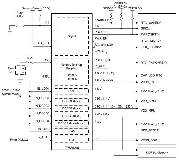
A. Block diagram shows TPS65218D0 powering AM437x processor. For TPS6521835, refer to this Tech Note. For TPS6521815, the wiring is not predefined and is programmed for the specific processor in the application.
