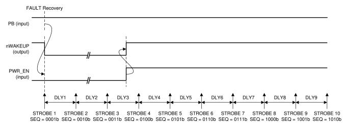
Figure 7-3. Power-Up Sequences from RECOVERY State
