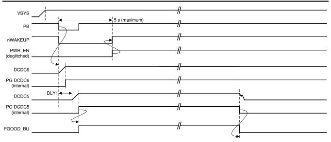
A. Sequence shown for TPS65218D0 and TPS6521825 variants. For TPS6521815 variant, order and timing of DCDC5 and DCDC6 can be modified using registers SEQ1-2 and SEQ5 in Section 7.5.4.
