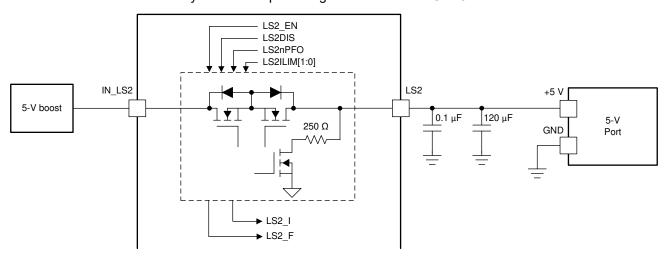
Figure 7-12. Typical Application of Load Switch 2
