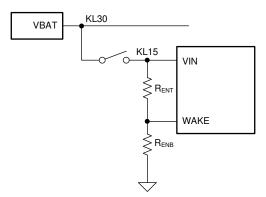
Figure 11-35. System UVLO by Enable Dividers
