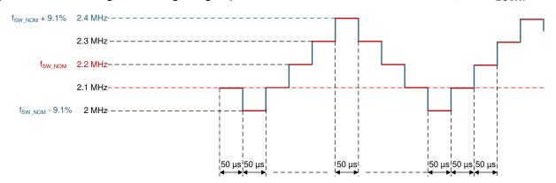
Figure 10-3. Modulated SYNC Input Clock (General Example With ±14% Variation and 100-kHz Steps)
