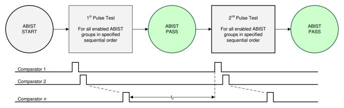
Figure 11-8. ABIST Delayed Test Pulses
