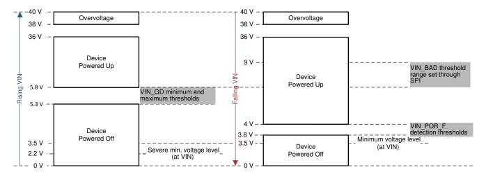
Figure 10-1. VIN Rising and Falling Ranges (With EXTSUP Supplied by VBOOST and V<sub>BUCK1</sub> = 3.3 V)
