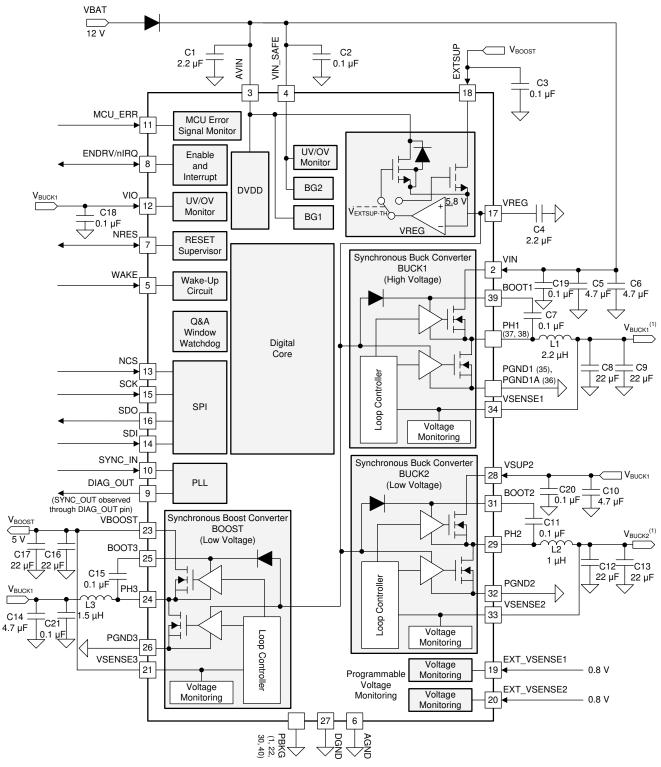
1. The VBUCK1 voltage is 3.3 V or 3.6 V. The VBUCK2 voltage is 1.2 V, 1.25 V, 1.8 V, or 2.3 V.
