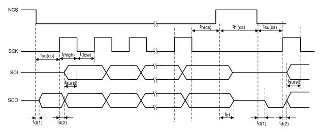
Figure 9-1. SPI Timing Parameters
