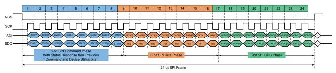
1. The SPI master device (MCU) and SPI slave device (TPS65313-Q1) sample the received data on the falling SCK edge and transmit data on the rising SCK edge.
