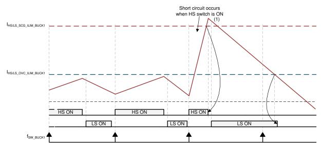
1. When the BUCK1 load current continues to increase to greater than the maximum specified load, an UV event can occur.
