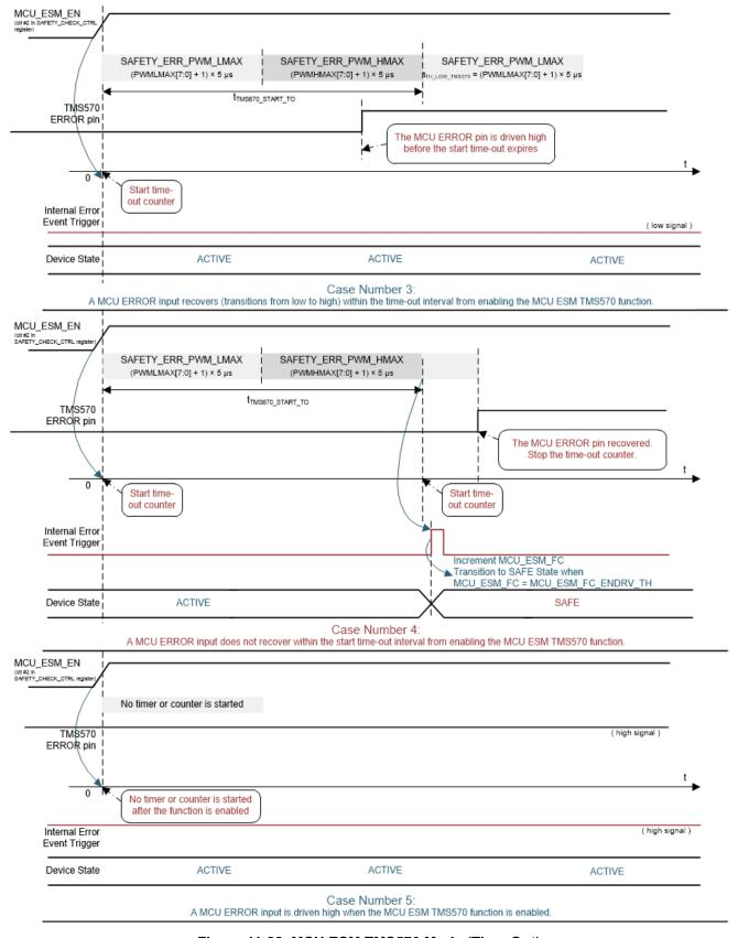
Figure 11-22. MCU ESM TMS570 Mode (Time-Out)
