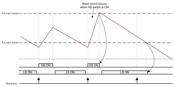
When the BUCK2 load current continues to increase to greater than the IBUCK2\_LOAD maximum value, an UV event can occur.
