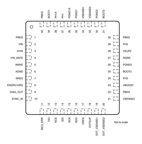
Figure 8-1. 40-Pin RWG VQFNP (Top View)
