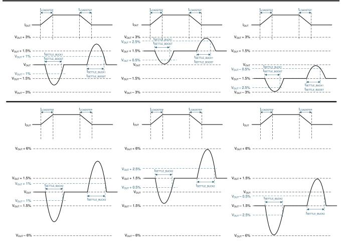
Figure 10-4. Regulator Load-Step Response
