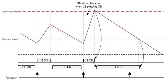
1. When the BOOST load current continues to increase to greater than the IBOOST\_LOAD maximum value, an UV event can occur.
