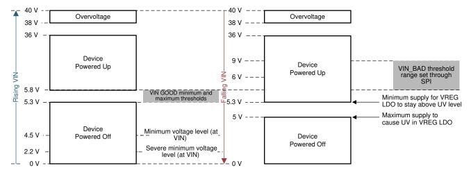
Figure 10-2. VIN Rising and Falling Ranges (With EXTSUP Not Present or Connected, and V<sub>BUCK1</sub> = 3.3 V)
