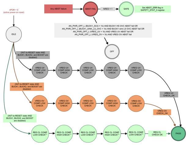
1. The regulator current-limit test (REG CL) includes the BUCK1, BUCK2, and BOOST current-limit circuits.
