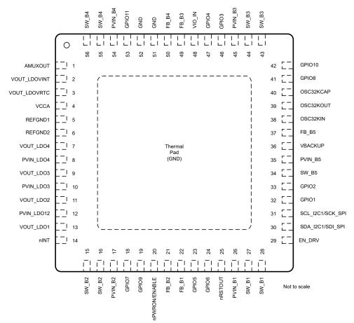
Figure 6-1. 56-Pin RWE (VQFNP) Package, 0.5-mm Pitch, With Thermal Pad (Top View)
