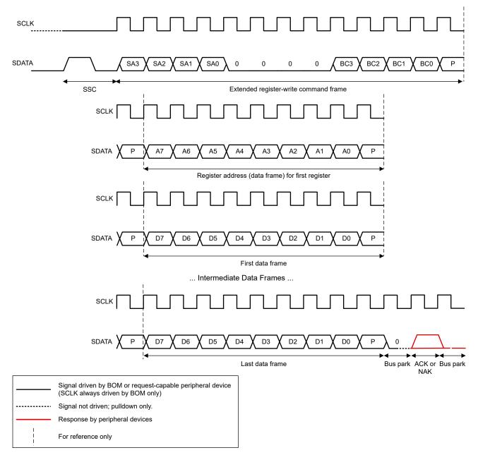
Figure 8-46. SPMI Extended Register Write Command
