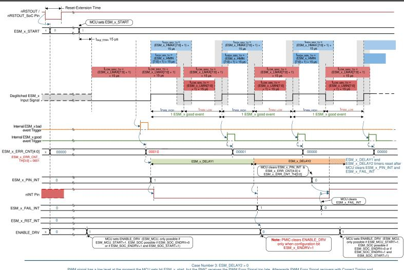
PWM signal has a low level at the moment the MCU sets bit ESM\_x\_start, but the PMIC receives the PWM Error Signal too late. Afterwards PWM Error Signal recovers with Correct Timing and ESM\_x\_ERR\_\_CNT[4:0] reaches a value less than the configured ESM\_x\_ERR\_\_CNT\_TH[3:0] before elapse of the ESM\_x\_DELAY2 time-interval
