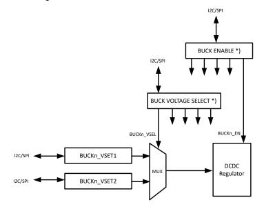
\*) BUCK ENABLE and BUCK VOLTAGE SELECT bits are located in BUCKx\_CTRL register
