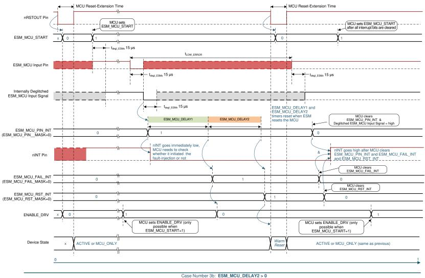
An error event occurred in the MCU, and the MCU is unable to correct the error before elapse of the ESM\_MCU\_DELAY1 and ESM\_MCU\_DELAY2 time-intervals. Hence the PMIC resets the MCU
