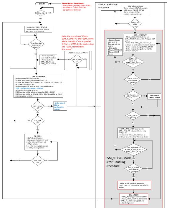
Figure 8-25. Flow Chart for Error Detection in Level Mode
