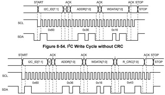
The I<sup>2</sup>C controller device (the MCU) provides R\_CRC[7:0], which is calculated from the I2C\_ID, R/W, ADDR, and the WDATA bits (24 bits). See CRC Calculation for I2C and SPI Interface Protocols.
