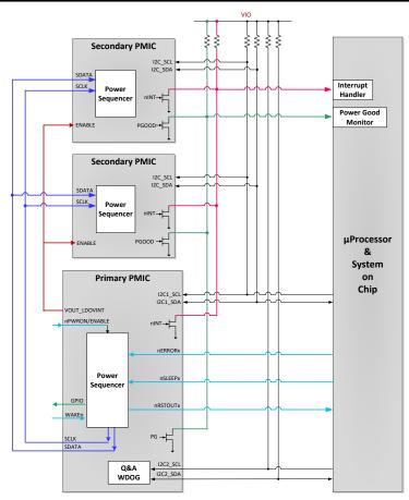
Figure 8-44. Multi-PMIC Pin Connections
