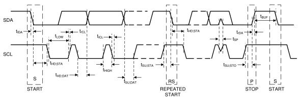
Figure 8-52. I<sup>2</sup>C-Compatible Timing
