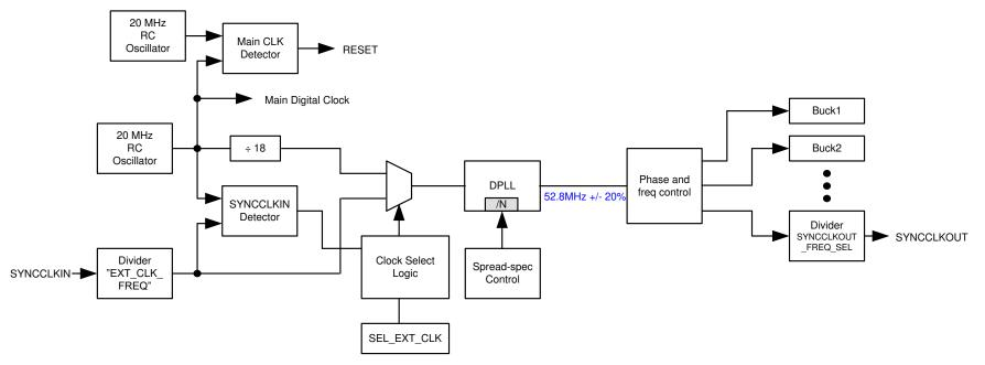
Figure 8-8. Sync Clock and DPLL Module
