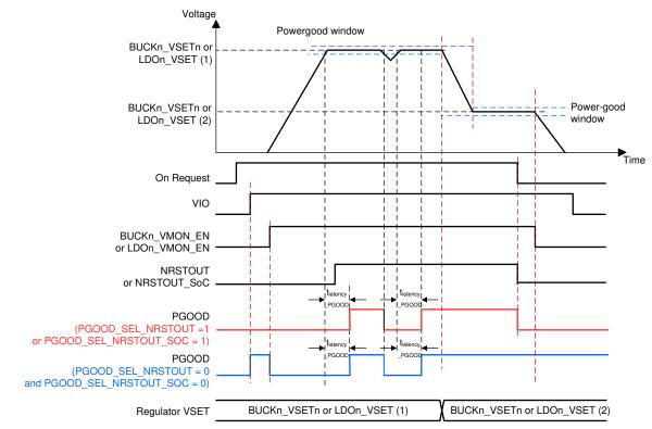
Figure 8-11. PGOOD Waveforms
