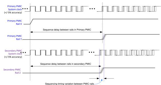
Figure 8-45. Multi-PMIC Rail Sequencing Timing Variation
