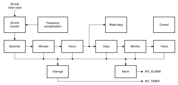
Figure 8-13. RTC Block Diagram
