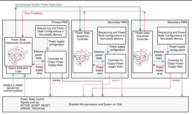
Figure 8-43. Multi-PMIC Power State Synchronization Block Diagram
