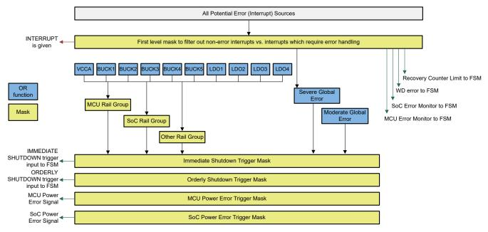
Figure 8-37. Error Source Hierarchical Mask System
