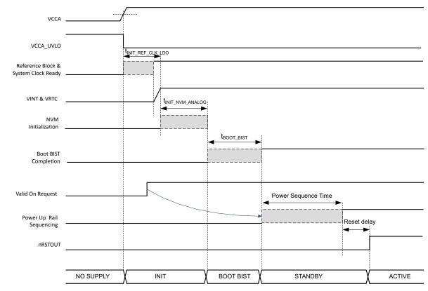
Figure 8-41 shows the timing diagram of the TPS6593-Q1 after the first supply detection.
