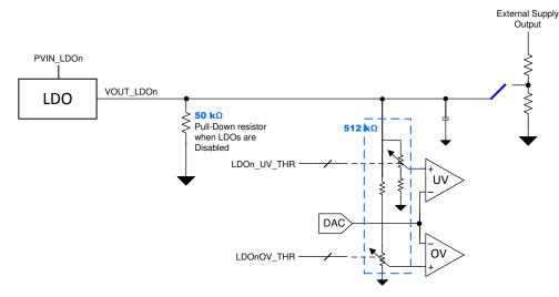
Figure 8-9. Impedance at the VOUT\_LDOn Pins
