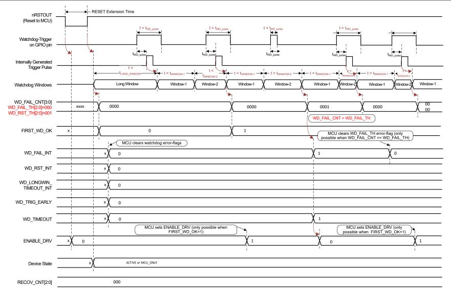
Figure 8-20. Watchdog in Trigger Mode – Good Events (Correct Watchdog-Triggers) After Start-up, Followed by a Bad-Event (No Watchdog-Trigger in Window-2) and After That Followed by a Good Event.
