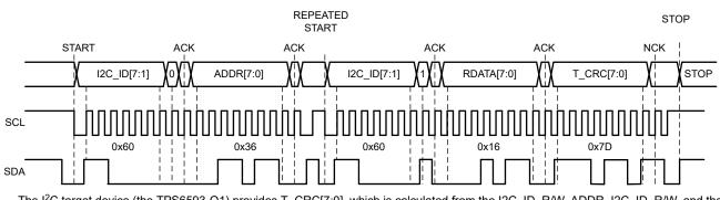
The I<sup>2</sup>C target device (the TPS6593-Q1) provides T\_CRC[7:0], which is calculated from the I2C\_ID, R/W, ADDR, I2C\_ID, R/W, and the RDATA bits (32 bits). See CRC Calculation for I2C and SPI Interface Protocols.
