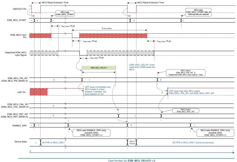
An error event occurred in the MCU, and the MCU is unable to correct the error before elapse of the ESM\_MCU\_DELAY1 time-interval. Hence the PMIC resets the MCU
