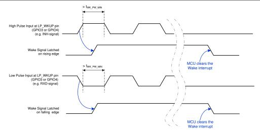
Figure 8-40. CAN Wake-Up Timing Diagram
