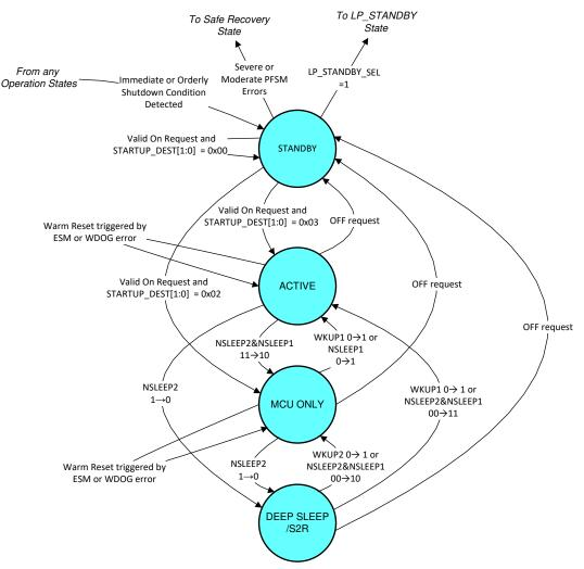
Figure 8-39. Example of a Mission State-Machine
