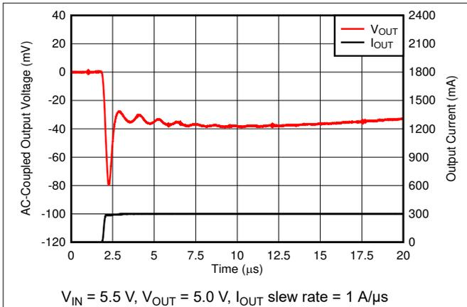
**Figure 6-19.  $I_{OUT}$  Transient From 1 mA to 300 mA**
