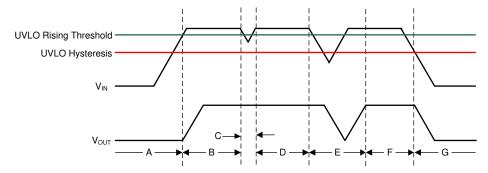
Figure 7-2. Typical UVLO Operation
