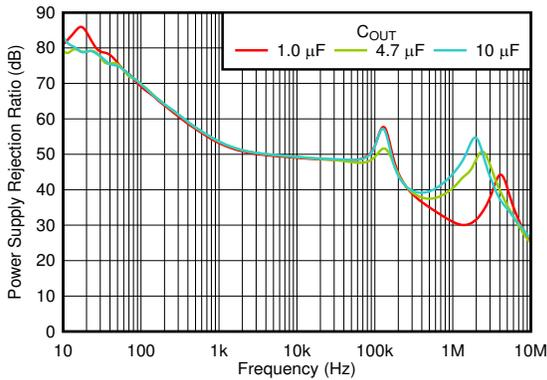
$V_{IN} = 4.3\text{ V}$ ,  $C_{IN} = 0\ \mu\text{F}$ ,  $V_{OUT} = 3.3\text{ V}$ ,  $I_{OUT} = 300\text{ mA}$
