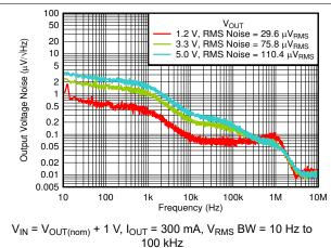
Figure 6-29. Output Noise vs Frequency and V<sub>OUT</sub>
