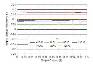
Output Accuracy vs I<sub>OUT</sub> for 5.0 V
