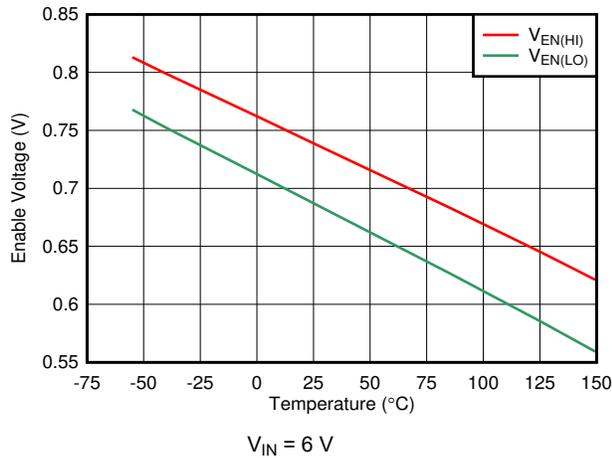
Figure 6-13.  $V_{EN(HI)}$  and  $V_{EN(LO)}$  Threshold vs Temperature
