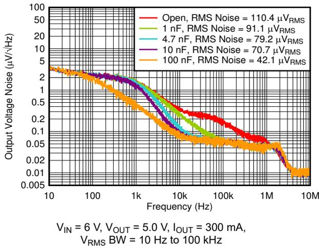
Figure 6-31. Output Noise vs Frequency and  $C_{FF}$
