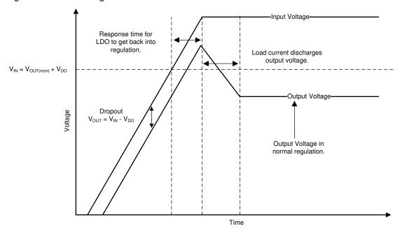
Figure 8-3. Start-Up Into Dropout
