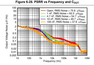
$V_{\text{IN}}$  = 4.3 V,  $V_{\text{OUT}}$  = 3.3 V,  $I_{\text{OUT}}$  = 300 mA,  $V_{\text{RMS}}$  BW = 10 Hz to 100 kHz
