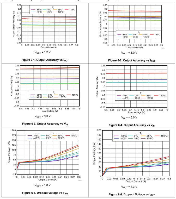
at operating temperature  $T_J$  = 25°C,  $I_{OUT}$  = 1 mA,  $V_{EN}$  = 1.0 V,  $C_{IN}$  = 1.0  $\mu$ F,  $C_{OUT}$  = 1.0  $\mu$ F, and  $V_{IN}$  =  $V_{OUT(NOM)}$  + 0.5 V or 1.65 V (whichever is greater), unless otherwise noted; typical values are at  $T_J$  = 25°C
