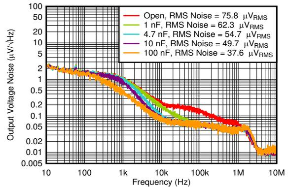
$V_{IN} = 4.3\text{ V}$ ,  $V_{OUT} = 3.3\text{ V}$ ,  $I_{OUT} = 300\text{ mA}$ ,  $V_{RMS}\text{ BW} = 10\text{ Hz to }100\text{ kHz}$
