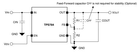
Figure 8-1. Output Voltage Setting
