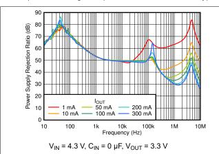
Figure 6-25. PSRR vs Frequency and I<sub>OUT</sub>
