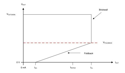
Figure 7-1. Foldback Current Limit
