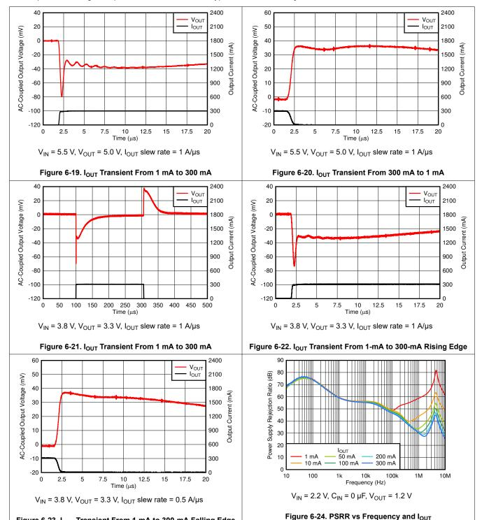
Figure 6-23. I<sub>OUT</sub> Transient From 1-mA to 300-mA Falling Edge
