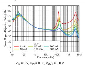
Figure 6-26. PSRR vs Frequency and I<sub>OUT</sub>
