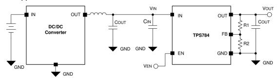
Figure 8-7. Operation From a DC/DC Converter
