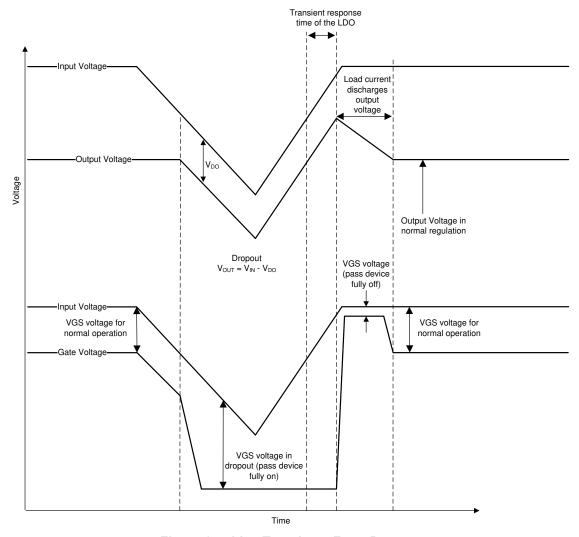
Figure 8-4. Line Transients From Dropout
