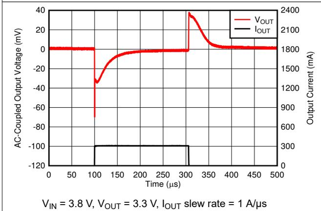
**Figure 6-21.  $I_{OUT}$  Transient From 1 mA to 300 mA**
