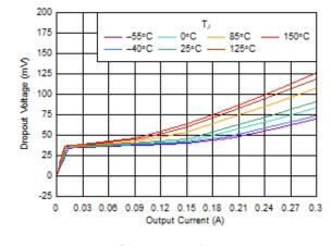
Dropout vs I<sub>OUT</sub>
