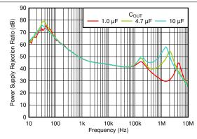
$V_{IN}$  = 6 V,  $C_{IN}$  = 0  $\mu$ F,  $V_{OUT}$  = 5.0 V,  $I_{OUT}$  = 300 mA
