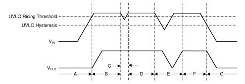
Figure 7-2. Typical UVLO Operation
