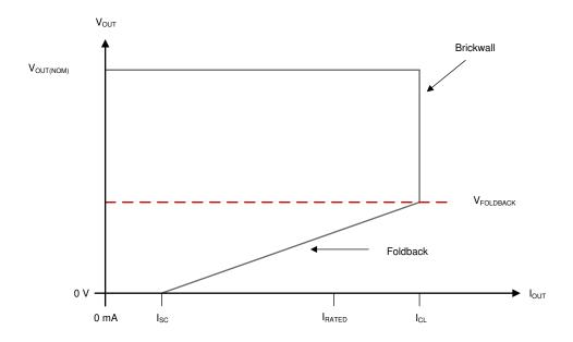
Figure 6-1. Foldback Current Limit
