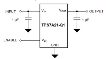
Figure 7-4. TPS7A21-Q1 Typical Application
