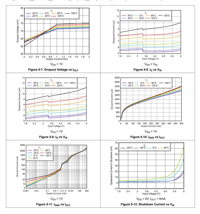
at  $V_{IN}$  = 3.6V,  $V_{OUT}$  = 3.3V,  $I_{OUT}$  = 1mA,  $C_{IN}$  = 1 $\mu$ F,  $C_{OUT}$  = 1 $\mu$ F, and  $T_A$  = 25°C (unless otherwise noted)
