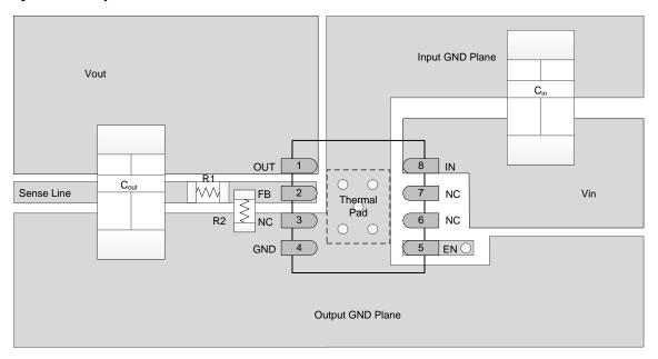
Figure 17. Recommended Layout Example
