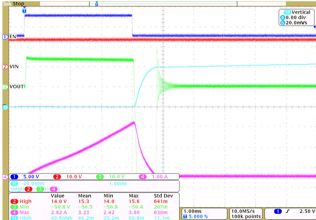
Figure 8-7. Inductive Load Switching-Off Waveform of 40mJ
