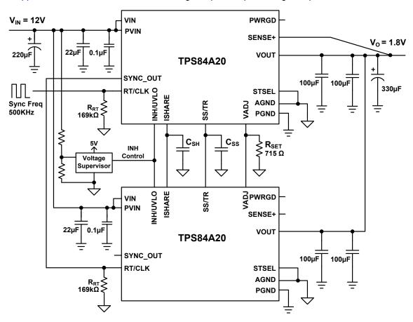
Figure 26. Typical TPS84A20 Parallel Schematic
