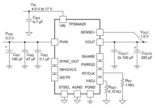
Figure 25. Typical Schematic PVIN = 3.3 V, VIN = 4.5 V to 17 V, VOUT = 1.0 V
