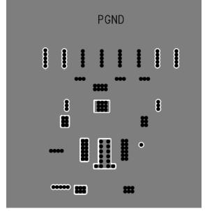
Figure 48. Typical Bottom-Layer Layout
