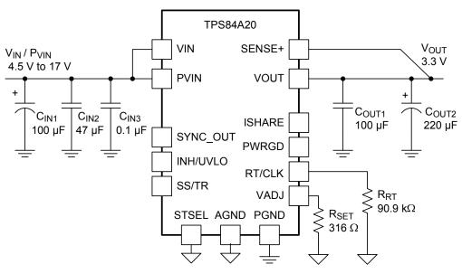
Figure 24. Typical Schematic PVIN = VIN = 4.5 V to 17 V, VOUT = 3.3 V
