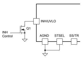
Figure 29. Typical Inhibit Control
