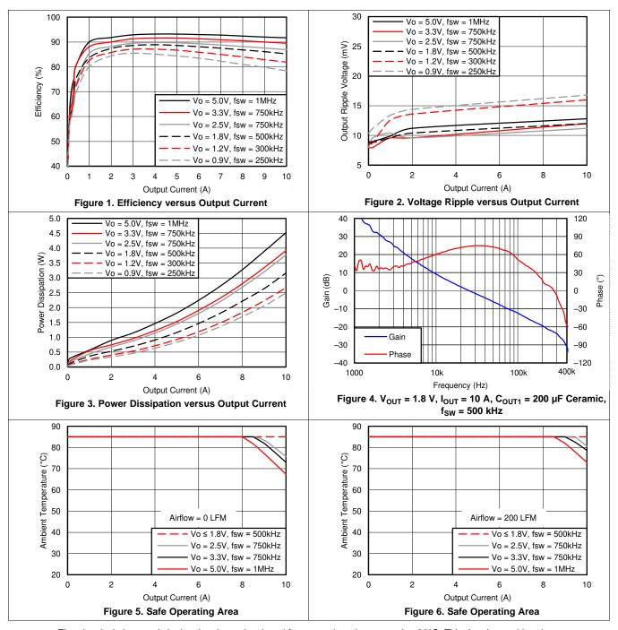
The electrical characteristic data has been developed from actual products tested at 25°C. This data is considered typical for the converter. Applies to Figure 1, Figure 2, and Figure 3.
