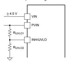
Figure 44. Adjustable PVIN Undervoltage Lockout, (VIN ≥4.5 V)
