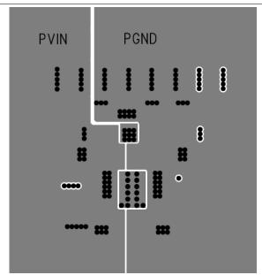
Figure 46. Typical Layer-2 Layout
