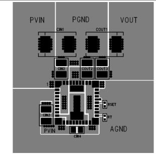
Figure 45. Typical Top-Layer Layout
