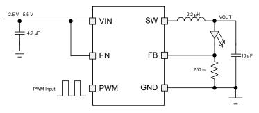
Figure 8-1. TPS92201 400 mA Output Application
