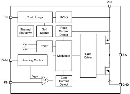
Figure 7-1. TPS92201 Functional Block Diagram
