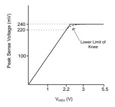
Figure 16. IADJ Pin Internal Clamp Characteristic
