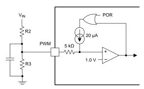
Figure 26. UVLO Programming Resistors
