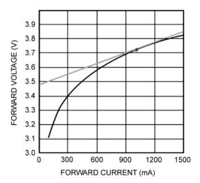
Figure 32. Calculating Dynamic Resistance r<sub>D</sub> from LED Specifications
