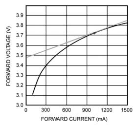
Figure 31. Calculating Dynamic Resistance r<sub>D</sub> from LED Characteristics.
