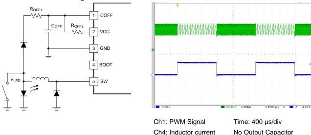
Figure 14. Shunt Dimming COFF Connection
