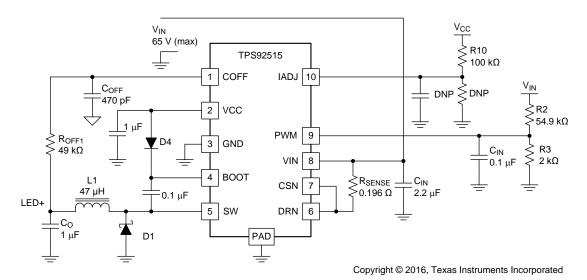
Figure 33. Application Schematic
