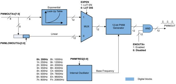
Figure 6-2. PWM Generator Path Diagram
