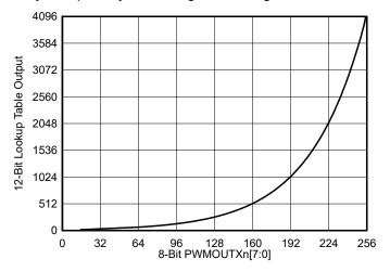
Figure 6-5. PWM Duty Cycle vs 8-Bit Code for Exponential Dimming
