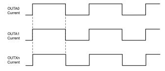
Figure 6-3. PWM Dimming Mode
