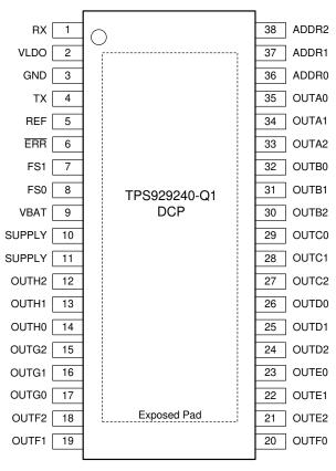
Figure 4-1. DCP Package 38-Pin HTSSOP with PowerPAD<sup>™</sup> Integrated Circuit Package Top View
