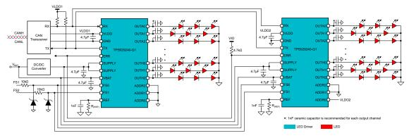
Figure 7-2. Typical Application Schematic
