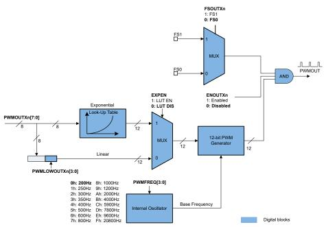
Figure 6-6. Output Current Control Path in FAIL-SAFE State
