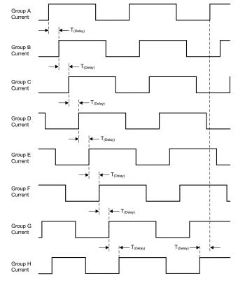
Figure 6-4. Phase Shift Dimming Mode
