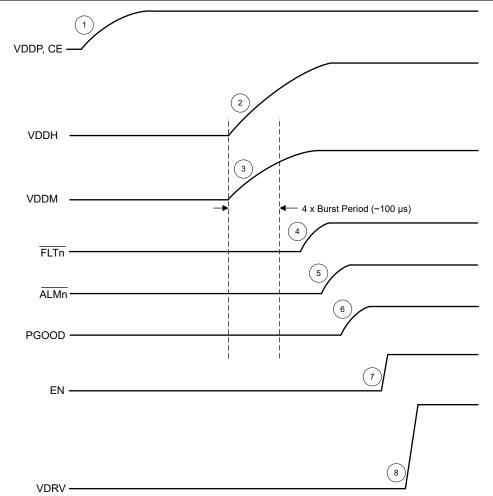
Figure 8-10. TPSI310x-Q1 Typical Start-up (CE = VDDP, FLTn\_CMP = 0, ALMn\_CMP = 0)
