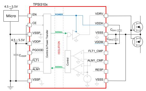
Figure 8-9. Simplified Schematic
