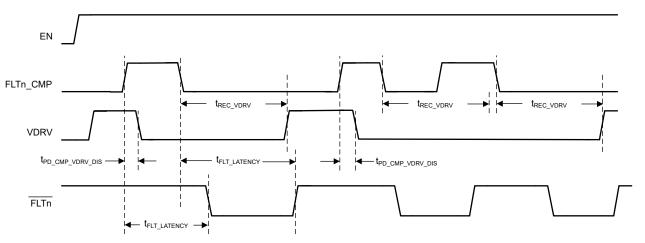
Figure 7-2. VDRV Auto-Recovery Timing (CE = 1 or CE = VDDP)
