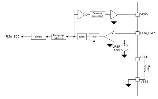
Figure 8-7. Latched Fault Comparator Block Diagram
