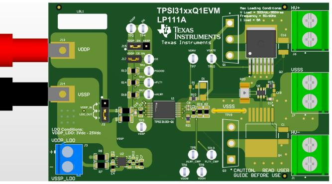
Figure 9-3. 3-D PCB View
