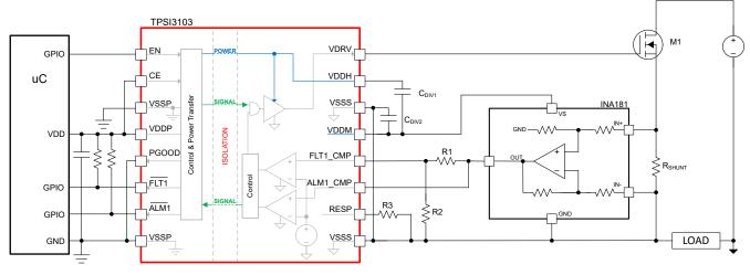
Figure 9-1. Typical Over-current Protection Application
