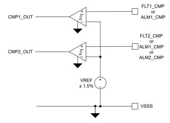
Figure 8-5. Comparator Block Diagram
