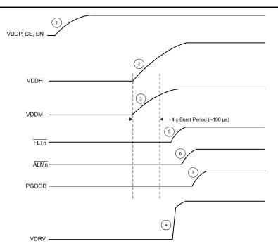
Figure 8-11. TPSI310x-Q1 Typical Start-up (CE = EN = VDDP, FLTn\_CMP = 0, ALMn\_CMP = 0)
