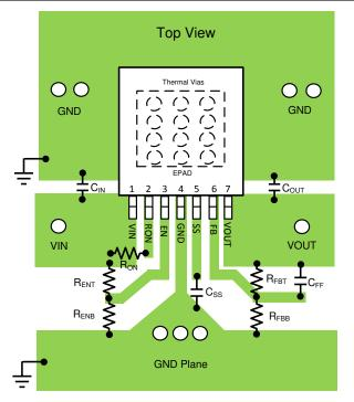
Figure 10-3. PCB Layout Guide
