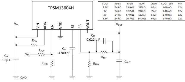
Figure 8-1. Simplified Application Schematic
