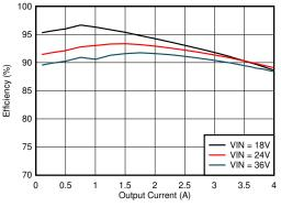
Efficiency  $V_{OUT}$  = 9.0 V,  $T_A$  = 25°C,  $F_{SW}$  = 300 kHz
