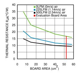
Figure 10-5. Package Thermal Resistance R<sub>0JA</sub> 4-Layer PCB with 1-oz Copper
