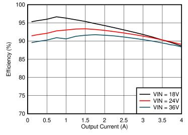
Figure 8-2. Efficiency  $V_{OUT}$  = 9.0 V,  $T_A$  = 25°C
