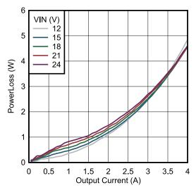
Figure 10-4. Power Dissipation V<sub>OUT</sub> = 9.5 V
