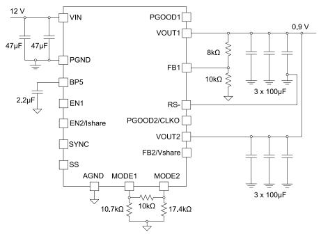
Figure 8-2. TPSM5D1806 Parallel Outputs Typical Schematic
