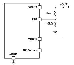
Figure 7-1. Single Device, Dual Output
