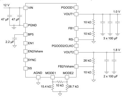
Figure 8-1. TPSM5D1806 Dual Output Typical Schematic
