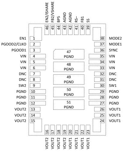
Figure 5-1. 51-Pin RDB QFN Package (Top View)
