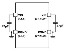
Figure 7-4. Input Capacitors Pin Connections
