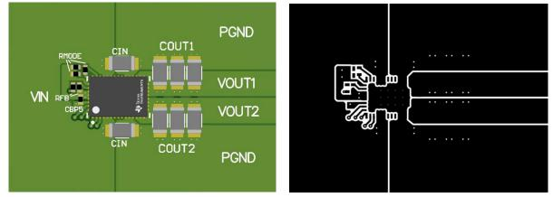
Figure 10-1. Typical Dual-Output Layout
