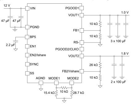
Figure 8-1. TPSM5D1806E Dual Output Typical Schematic
