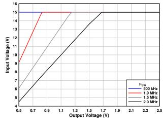
Figure 7-3. Maximum Input Voltage
