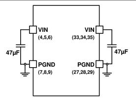
Figure 7-4. Input Capacitors Pin Connections
