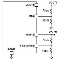
Figure 7-1. Single Device, Dual Output
