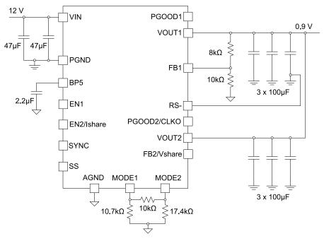
Figure 8-8. TPSM5D1806E Parallel Outputs Typical Schematic
