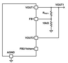
Figure 7-2. Single Device, Current Sharing
