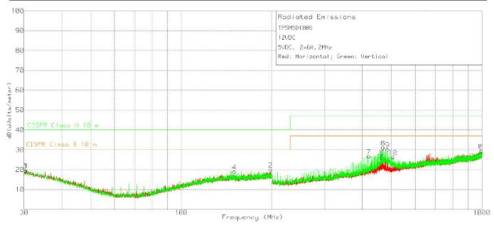
Figure 10-4. Radiated Emissions 12-V Input, 5-V Output, 6-A/Output Load
