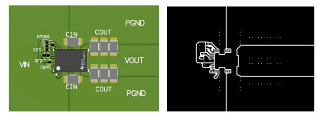
Figure 10-2. Typical Parallel-Output Layout
