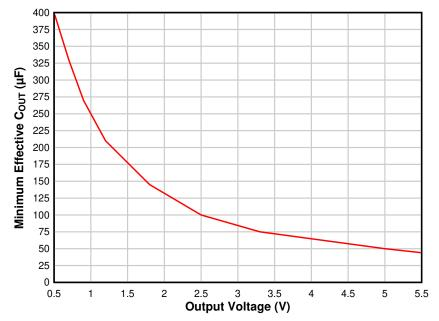
Figure 7-5. Minimum Required Output Capacitance (per Phase)
