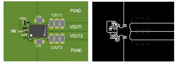
Figure 10-1. Typical Dual-Output Layout
