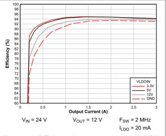
Figure 7-8. Efficiency improvements with VLDOIN (VOUT = 5 V)
