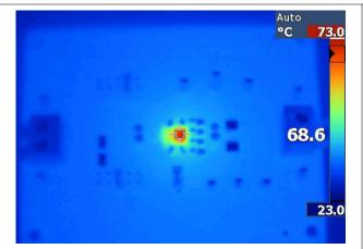
Figure 8-8. Thermal Image  $V_{IN}$  = 12 V,  $V_{OUT}$  = 3.3 V,  $F_{SW}$  = 1 MHz,  $I_{OUT}$  = 3 A
