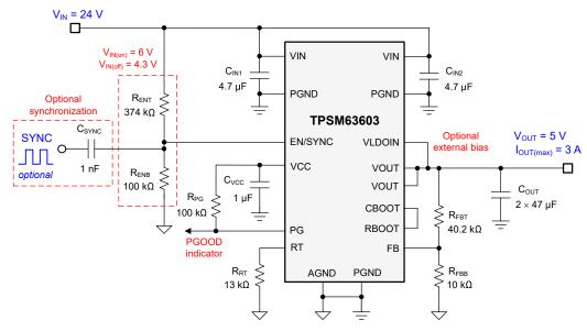
Figure 8-1. Circuit Schematic
