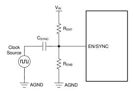
Figure 7-4. Typical Synchronization Using the EN/SYNC Pin
