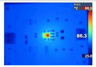
Figure 8-11. Thermal Image  $V_{IN}$  = 24 V,  $V_{OUT}$  = 5 V,  $F_{SW}$  = 1 MHz,  $I_{OUT}$  = 3 A
