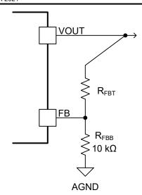
Figure 7-2. FB Resistor Divider
