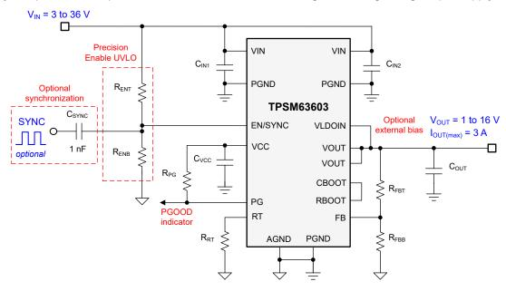
Figure 7-1. TPSM63603 Schematic Diagram with Input Voltage Operating Range of 3 V to 36 V
