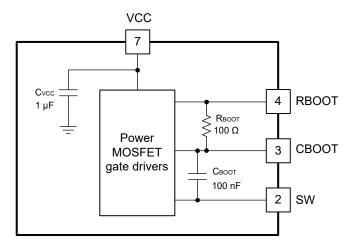
Figure 7-7. Internal BOOT Resistor
