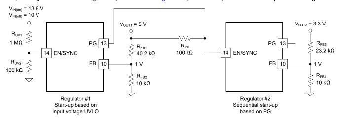
Figure 7-6. TPSM63603 Sequencing Implementation Using PG and EN/SYNC
