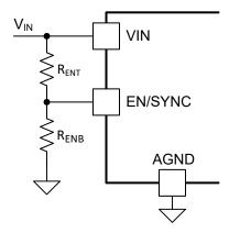
Figure 7-3. VIN UVLO Using the EN/SYNC Pin
