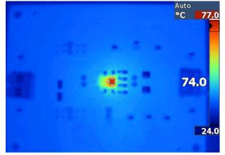
Figure 8-9. Thermal Image  $V_{IN}$  = 12 V,  $V_{OUT}$  = 5 V,  $F_{SW}$  = 1 MHz,  $I_{OUT}$  = 3 A
