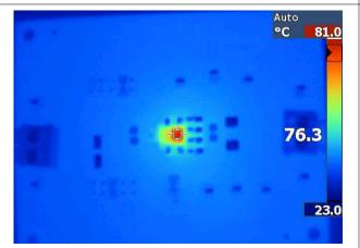
Figure 8-10. Thermal Image  $V_{IN}$  = 24 V,  $V_{OUT}$  = 3.3 V,  $F_{SW}$  = 1 MHz,  $I_{OUT}$  = 3 A
