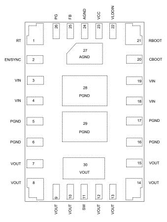
Figure 5-1. 30-Pin QFN, RDH Package (Top View)
