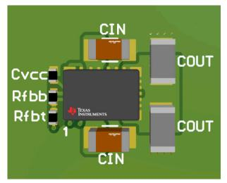
Figure 10-1. Typical Top-Layer Layout
