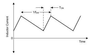
Figure 7-1. Continuous Conduction Mode (PWM-CCM) Current Waveform
