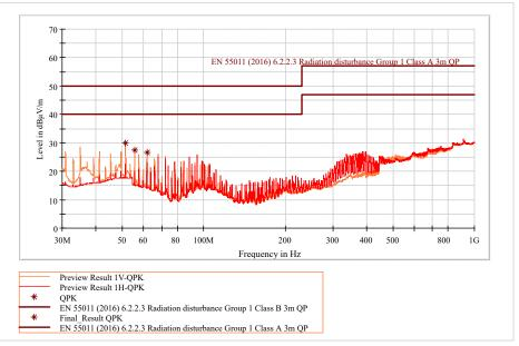
The above plot is measured on the EVM with the TPSM828303ARDSR and standard BOM.
