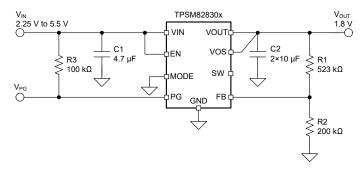
Figure 8-1. Typical Application of TPSM82830x
