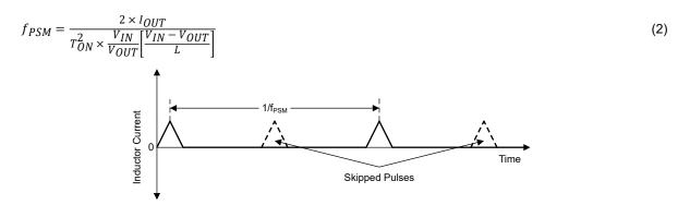
Figure 7-2. Discontinuous Conduction Mode (PSM-DCM) Current Waveform
