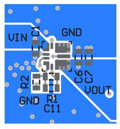
Figure 8-60. PCB Layout Recommendation (RDS Package)
