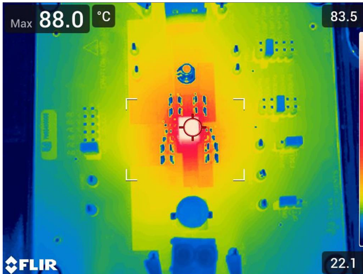
Figure 8-18. Thermal Image at 25^{\circ}\text{C} Ambient
