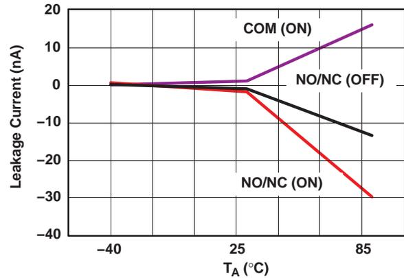
Figure 4. Leakage Current vs Temperature ( $V_+ = 3.3$  V)
