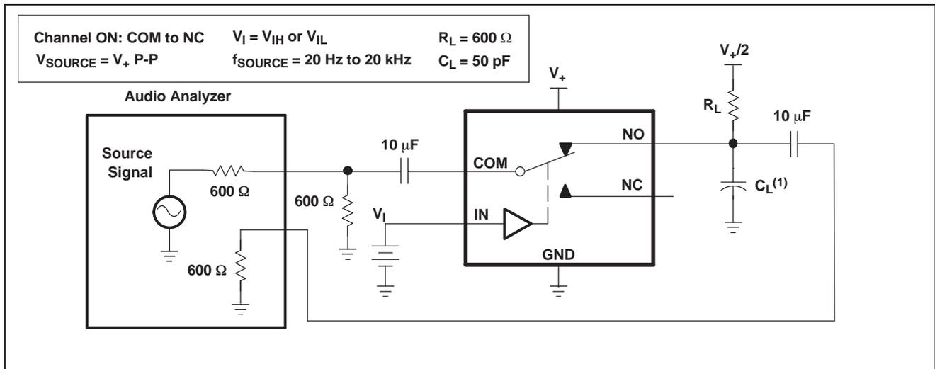
(1)  $C_L$  includes probe and jig capacitance.
