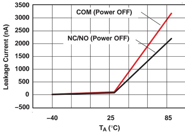
Figure 5. Leakage Current vs Temperature ( $V_+ = 5$  V)
