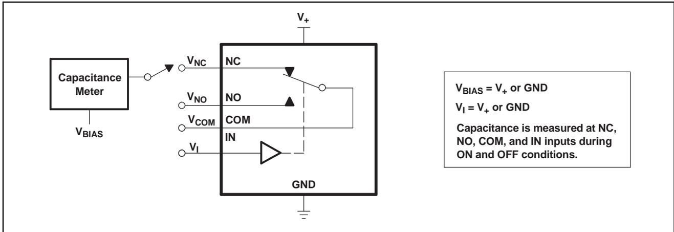
Figure 17. Capacitance ( $C_I$ ,  $C_{COM(ON)}$ ,  $C_{NC(OFF)}$ ,  $C_{NO(OFF)}$ ,  $C_{NC(ON)}$ ,  $C_{NO(ON)}$ )
