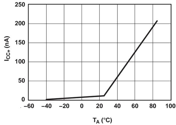
Figure 13. Current vs Temperature ( $V_+ = 5$  V)
