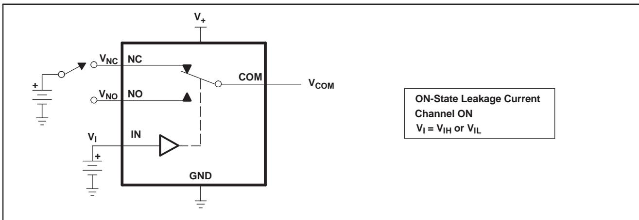
**Figure 16. ON-State Leakage Current ( $I_{COM(ON)}$ ,  $I_{NC(ON)}$ ,  $I_{NO(ON)}$ )**
