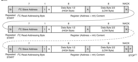
NOTES: (1) In order to start the next sequence, a STOP condition must be followed by a START condition. If no STOP is used, then a Repeated START must be used. Also note that is a STOP condition is issued in High-Speed mode, the mode will revert to the previous mode: Fast or Standard.
