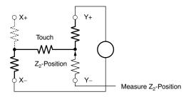
Figure 26. Pressure Measurement
