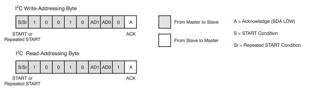
Figure 34. I<sup>2</sup>C Bus Addressing (Slave Address Byte Format)
