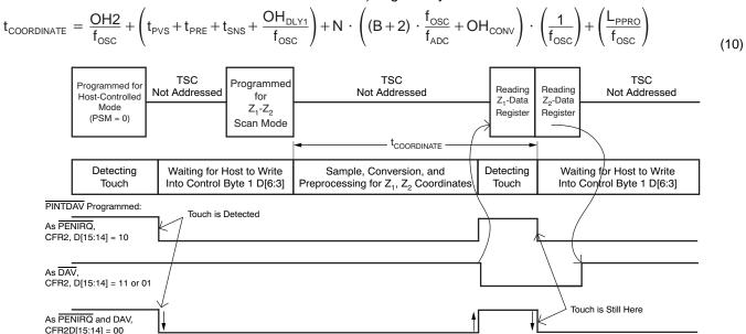
Figure 44. Example of a Z<sub>1</sub> and Z<sub>2</sub> Coordinate Touch Screen Scan (with Panel Stabilization Time) using TSMode 3
