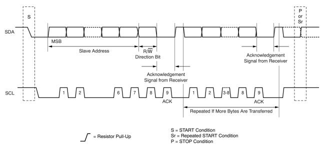
Figure 32. Complete Fast- or Standard-Mode Transfer
