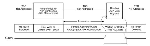
Figure 46. Non-Touch Screen, Non-Continuous AUX Measurement
