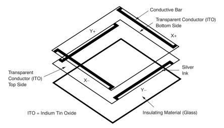
Figure 25. 4-Wire Touch Screen Construction
