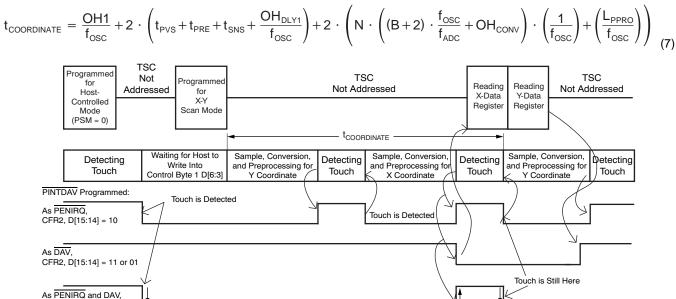
Figure 41. Example of an X and Y Coordinate Touch Screen Scan using TSMode 2
