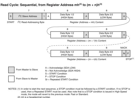
Figure 36. Sequential Read Cycle
