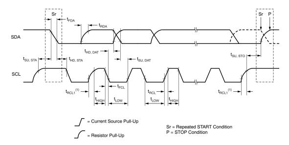
NOTE: (1) First rising edge of the SCL signal after Sr and after each acknowledge bit.
