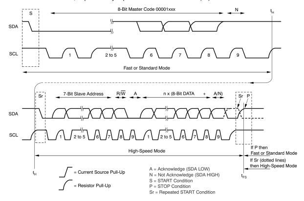
Figure 33. Complete High-Speed Mode Transfer
