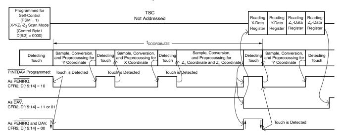
Figure 40. Example of an X, Y, and Z Coordinate Touch Screen Scan using TSMode 1
