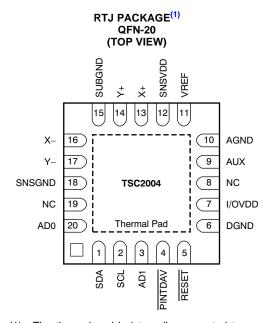
(1) The thermal pad is internally connected to SUBGND. The thermal pad can be connected to the analog ground or left floating. Keep the thermal pad separate from the digital ground, if possible.
