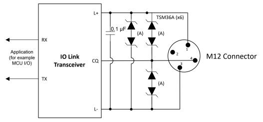
A. Diagram shows two TSM36A unidirectional devices stacked in series with the anodes tied back-to-back to protect between the respective signals.
