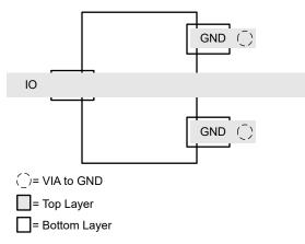
Figure 10-1. Routing with DBZ Package
