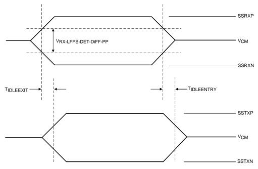
Figure 1. Idle Entry and Exit Latency
