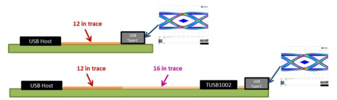
Figure 16. Linear Equalizer
