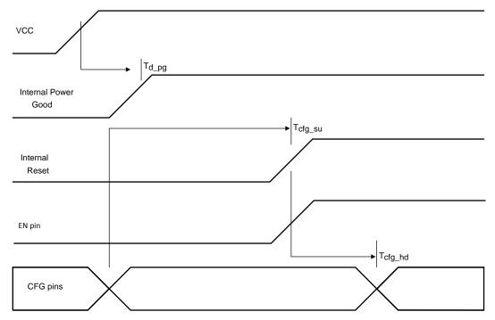
Figure 2. Power-Up Diagram
