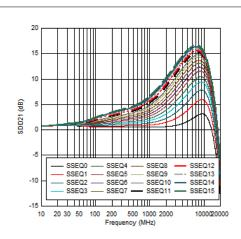
Figure 5-2. USB SSTX EQ Settings Curves at 85  $\Omega$  (from simulation)
