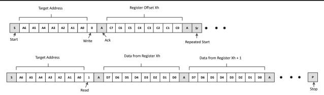
Figure 7-4. I2C Read with Repeated Start
