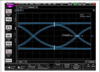
Figure 12-2. 10 Gbps Output Eye at CTX1 After 1.2 dB at 5 GHz Post-Channel
