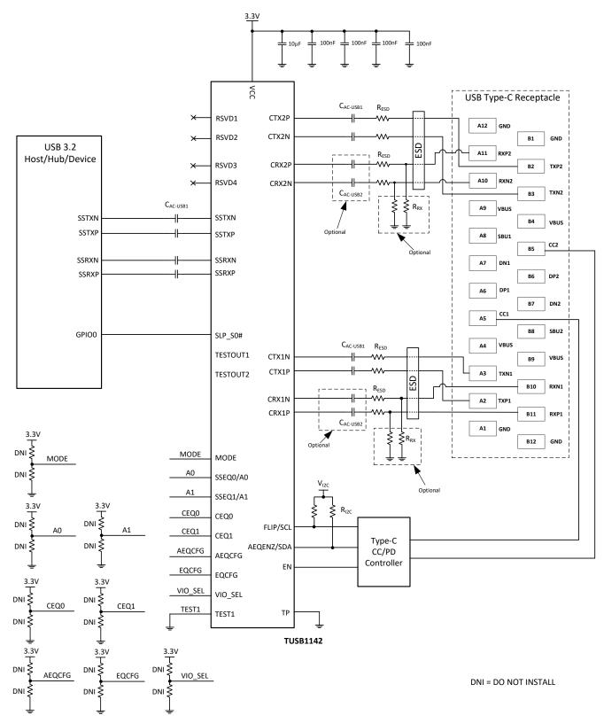
Figure 11-1. Application Circuit
