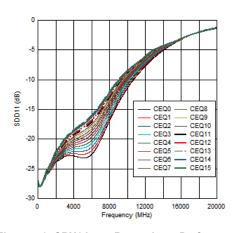
Figure 5-3. CRX1 Input Return Loss Performance at 85  $\Omega$  (from simulation)
