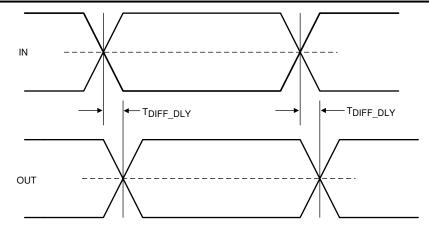
Figure 6-3. USB Propagation Delay
