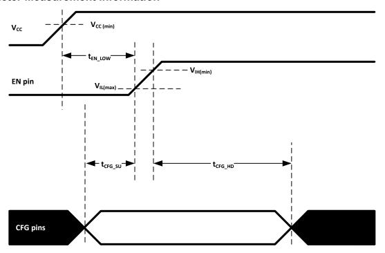
Figure 6-1. Power-On Timing Requirements
