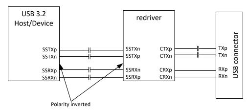
Figure 7-1. Polarity Inversion Example
