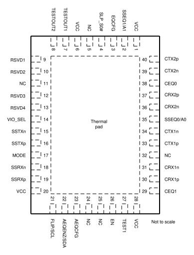
Figure 4-1. TUSB1142 RNQ Package, 40-Pin WQFN (Top View)
