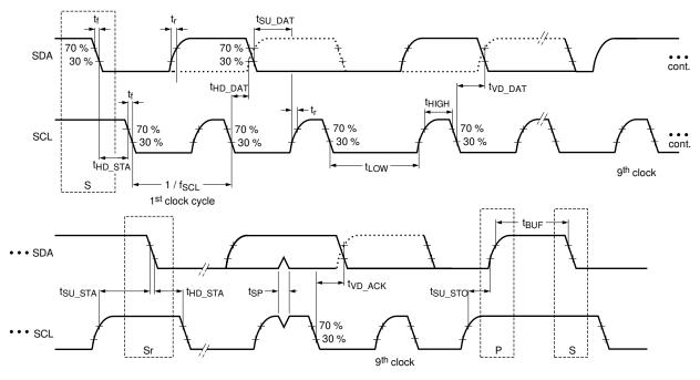
Figure 6-2. I2C Timing Diagram Definitions
