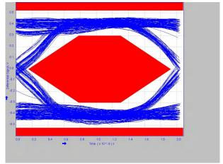
Figure 7-7. 5 Meter Pre-Channel With TUSB211A-Q1 EQ=2
