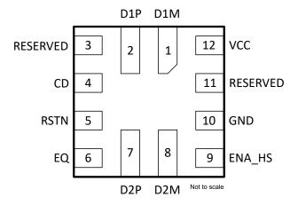
Figure 4-1. TUSB211A-Q1 RWB 12-Pin X2QFN (Top View)
