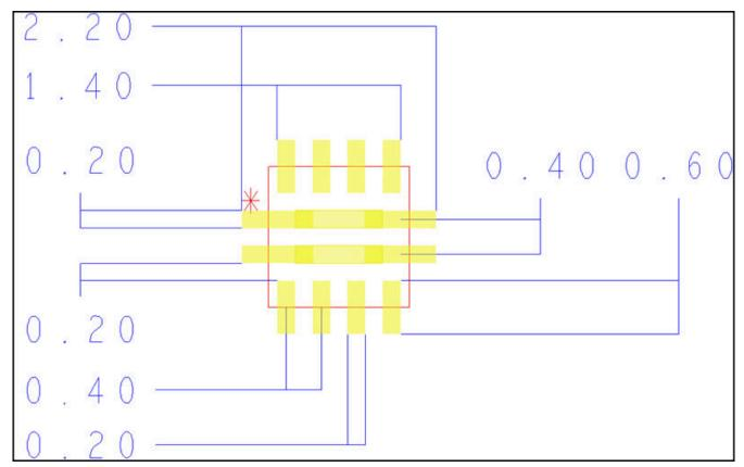
Figure 7-15. DP and DM Routing Underneath Device Package
