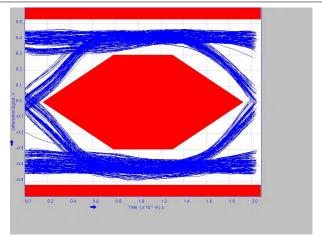
Figure 5-2. 5 Meter Pre-Channel With TUSB211A-Q1 EQ=2
