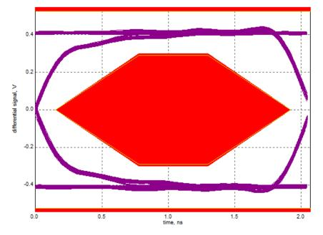
Figure 9-2. Typical USB 2.0 High Speed Eye Diagram
