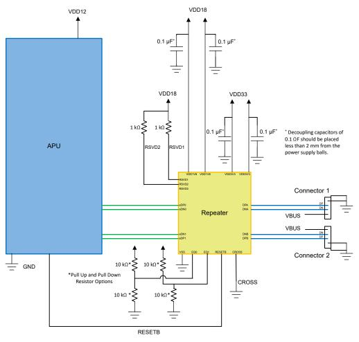
Figure 9-1. Typical Dual Port System Implementation
