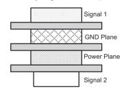
Figure 9-3. Four-Layer Board Stack-Up
