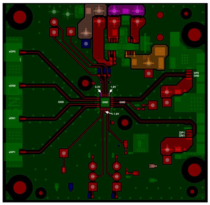
Figure 9-5. VQFN Example Layout
