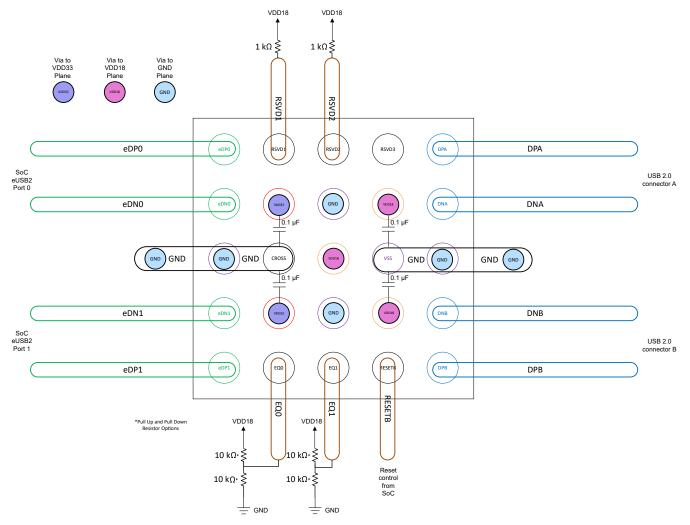
Figure 9-4. Example Layout of Application With No Cross MUX Function
