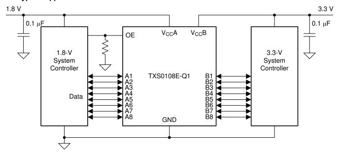
Figure 8-1. Typical Application Circuit
