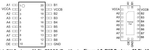
Figure 4-1. PW Package, 20-Pin TSSOP (Top View) Figure 4-2. RKS Package, 20-Pin VQFN (Top View)
