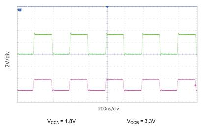
Figure 8-2. Level-Translation of a 2.5MHz Signal
