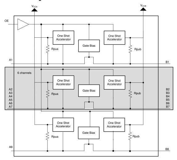
Each A-port I/O has a pull-up resistor ( $R_{PUA}$ ) to  $V_{CCA}$  and each B-port I/O has a pull-up resistor ( $R_{PUB}$ ) to  $V_{CCB}$ .  $R_{PUA}$  and  $R_{PUB}$  have a value of  $40k\Omega$  when the output is driving low.  $R_{PUA}$  and  $R_{PUB}$  have a value of  $4k\Omega$  when the output is driving high.  $R_{PUB}$  are disabled when OE = Low.
