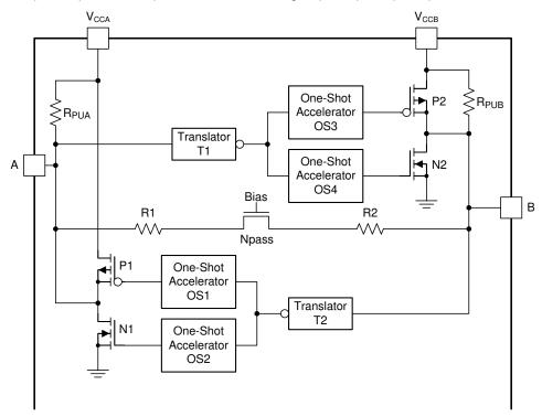
Figure 7-1. Architecture of a TXS0108E-Q1 Cell
