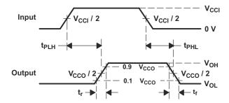
Figure 6-5. Propagation Delay Times
