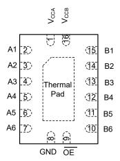
Figure 4-1. BQB Package, 16-Pin WQFN (Top View)
