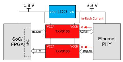
Figure 8-5. Using the TXV0106 for Power Isolation
