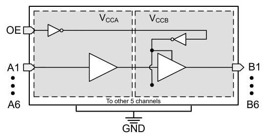
Figure 7-1. Functional Block Diagram of the TXV0106
