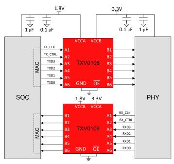
Figure 8-1. RGMII Application (Interfacing between MAC and PHY)
