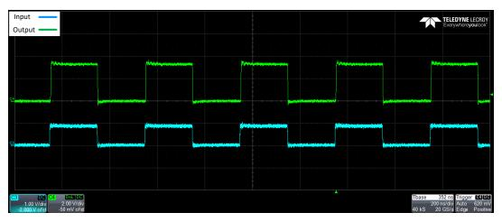
Figure 8-2. Up Translation (1.8V to 3.3V) C<sub>LOAD</sub> = 15pF at 2.5MHz
