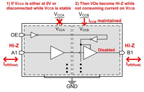
Figure 7-2. V<sub>CC</sub> Disconnect and V<sub>CC</sub> Isolation Feature
