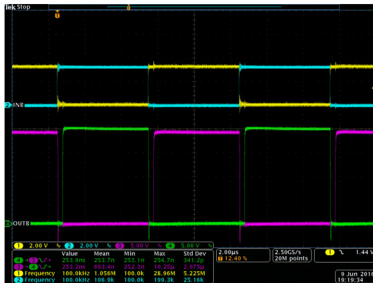
Figure 8-5. Bench Test Waveform for INA/B and OUTA/B
