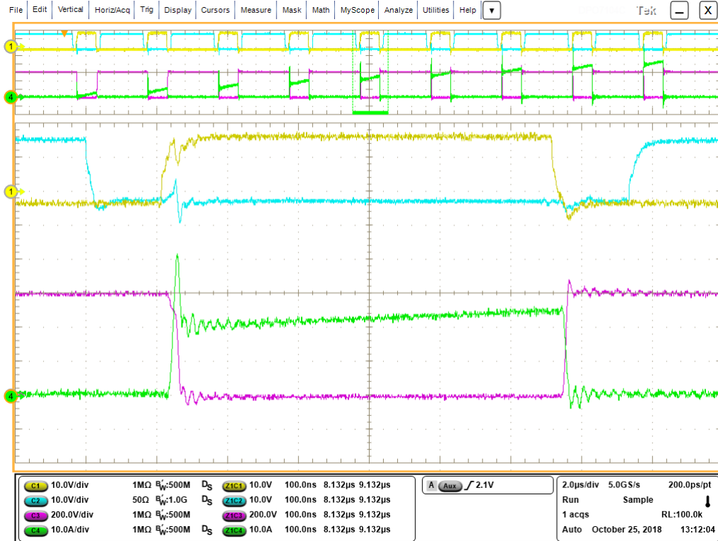
Figure 9-6. SiC MOSFET Switching Waveforms
