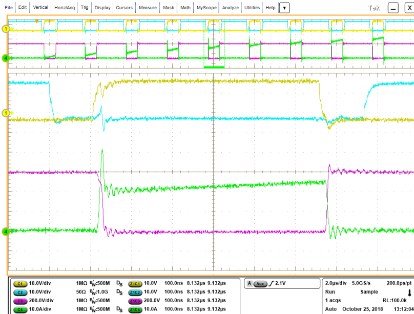
Figure 8-6. SiC MOSFET Switching Waveforms
