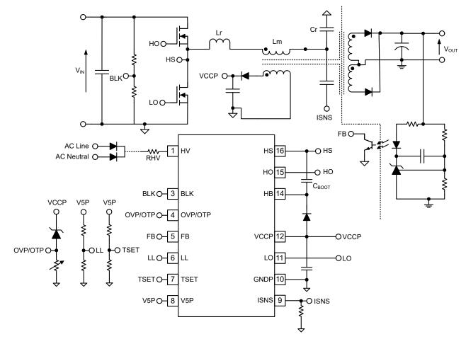
Figure 7-1. Simplified Application Schematic
