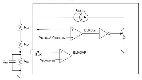
Figure 7-6. BLK Pin Input Voltage Sensing Architecture
