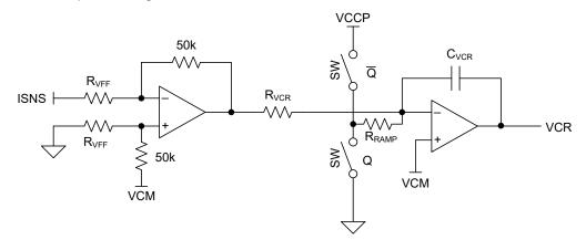
Figure 7-3. VCR Synthesizer Block Diagram
