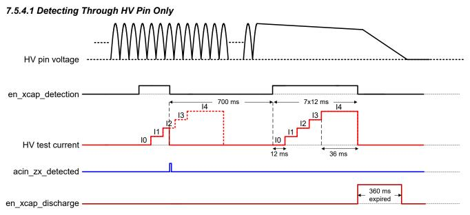
Figure 7-21. Zero Cross Detection Sequence HV Pin Only
