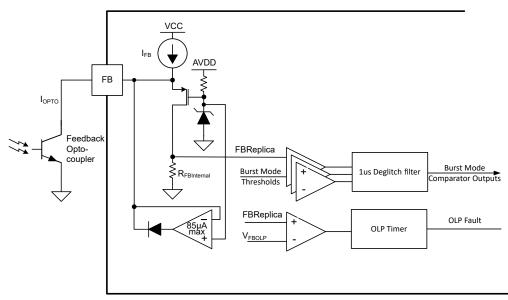
Figure 7-4. Feedback Chain Block Diagram
