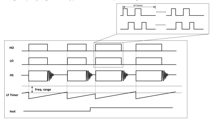
Figure 7-18. Packet Size Regulation Inside LF Burst
