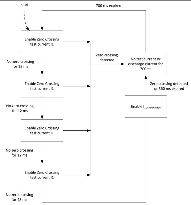
Figure 7-22. AC ZCD and X-Capacitor Discharge Flow Chart
