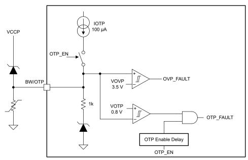
Figure 7-7. mOVP/OTP Protection Architecture
