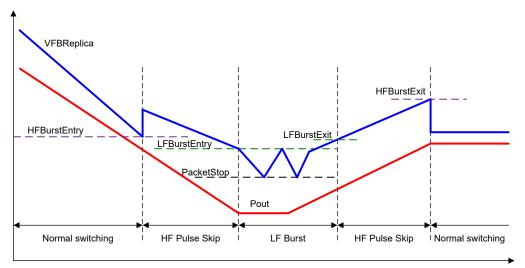
Figure 7-19. Burst Mode Determination from FBReplica Comparators
