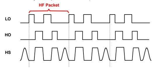
Figure 7-16. High Frequency Pulse Skip Packet
