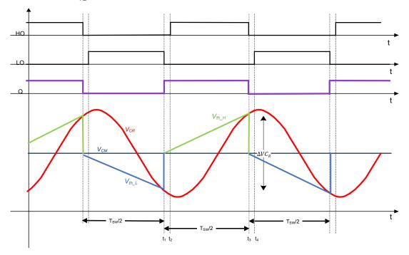
Figure 7-2. IPPC Basic waveforms
