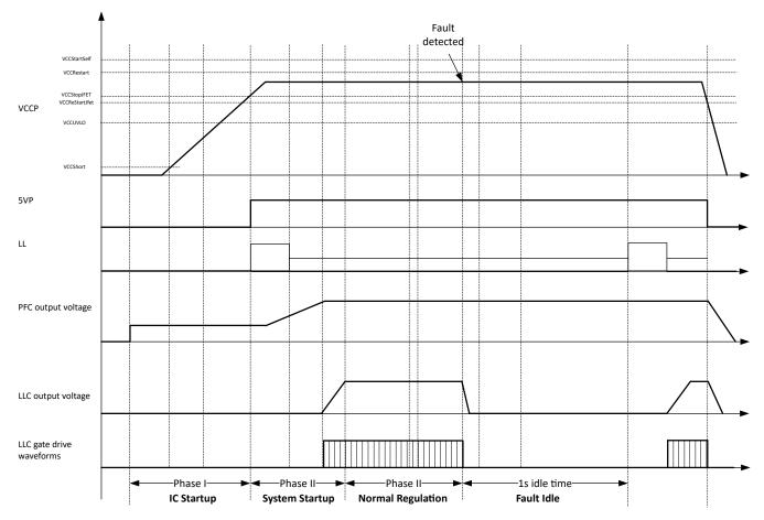
Figure 7-14. Startup Sequence for "HV Startup" Feature Disabled
