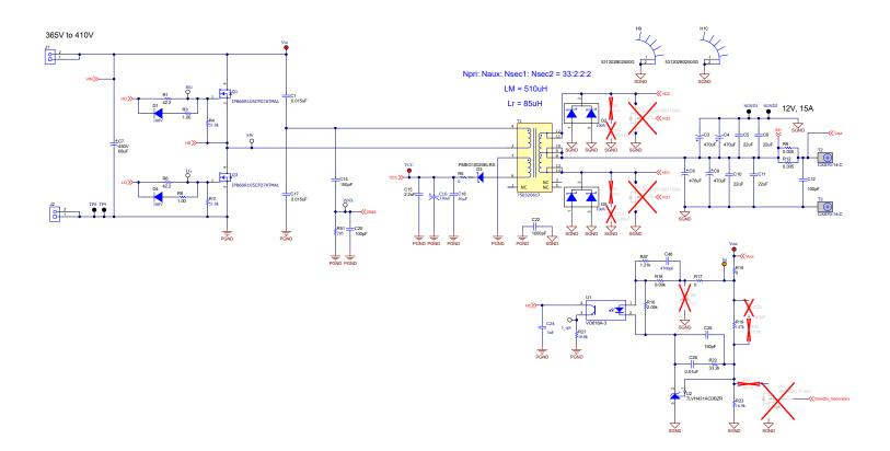
Figure 8-5. UCC25660EVM-064 Power Stage Schematic
