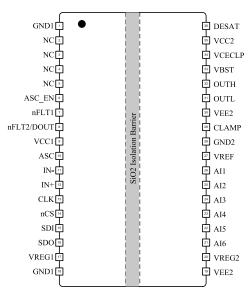
Figure 5-1. DWJ 36-Pin SOIC Top View
