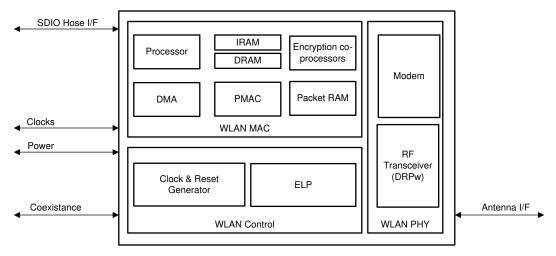
Figure 4-1. WL18x1 High-Level Wi-Fi System Diagram
