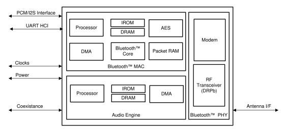
Figure 4-2. WL1831 High-Level Bluetooth System Diagram
