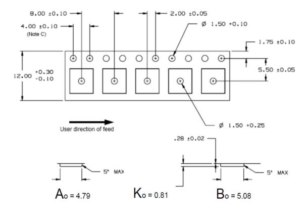
NOTES : A. Tolerance unless otherwise specified : ± 0.10. B. Unless otherwise noted, R = 0.3 MAX. C. 10 pitch cumulative tolerance : ± 0.20.
