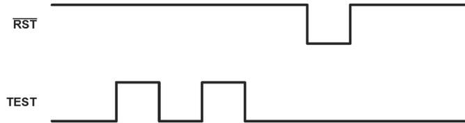
Note: This toggling of TEST pins is not subject to timing constraints. The appropriate level transitions on TEST pin, followed by a RST pulse after 50us, are sufficient to trigger an exit from BSL mode.
