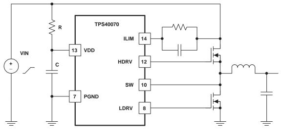
Figure 1. Limiting the Slew Rate
