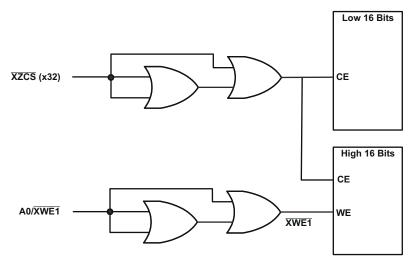
Figure 4-3. Example Delay Line Circuit
