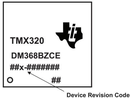
Figure 1. Example 1, Device Markings for TMX320DM368 (ZCE)
