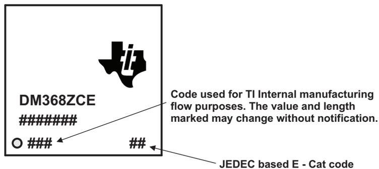
Figure 2. Example 2, Device Markings for TMS320DM368 (ZCE)
