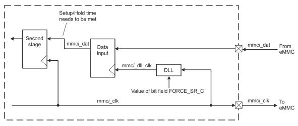
Figure 2-1. Simplified SoC 192-MHz Mode DLL Block Diagram
