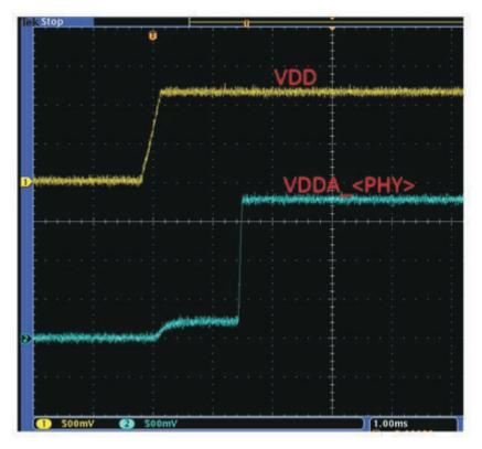
Figure 4-2. Leakage Voltage
