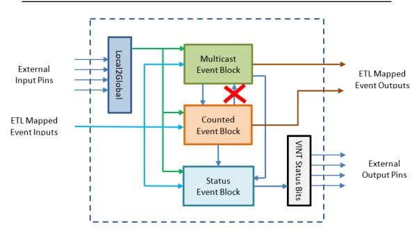
Figure 2-3. Interrupt Aggregator Version 1.0
