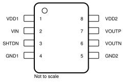
Figure 2. Pin Diagram
