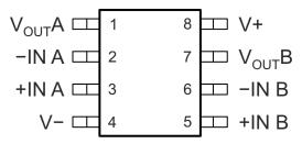
Figure 3-1. Pin Diagram
