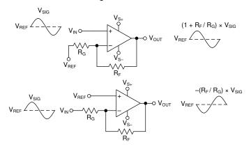
Figure 1-1. Functional Block Diagram
