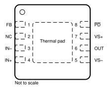
Figure 3-1. Pin Diagram
