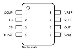
Figure 4-1. Pin Diagram SOIC (8) and VSSOP (8) Packages
