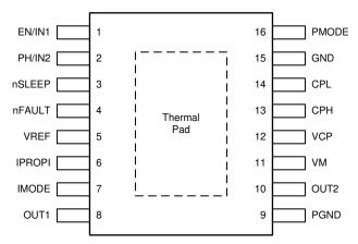
Figure 4-1. DRV8876-Q1 Pin Diagram
