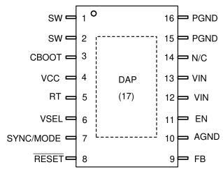
Figure 4-1. Pin Diagram for HTSSOP
