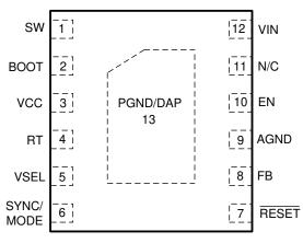
Figure 4-2. Pin Diagram for WSON
