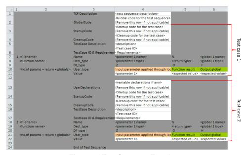
Figure 14. Test Sequence Template
