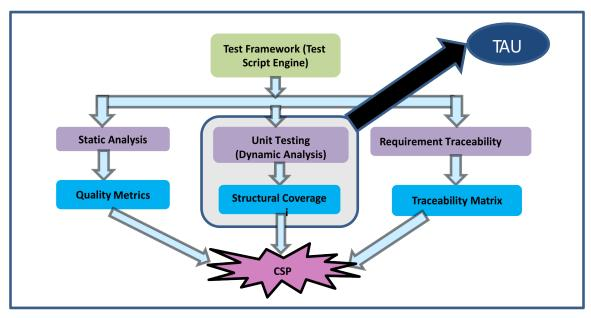
Figure 3. Test Automation Framework for CSP
