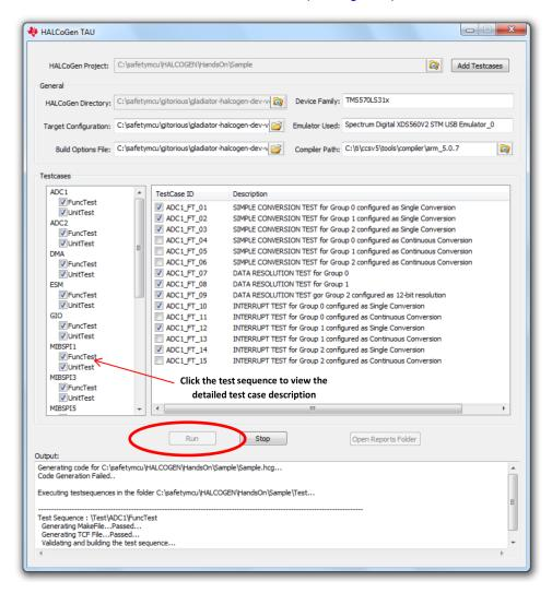
Figure 9. Test Case Selection and Run
