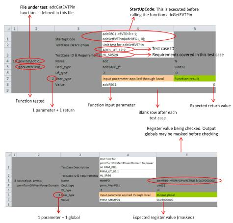
Figure 16. Examples of a Test Case
