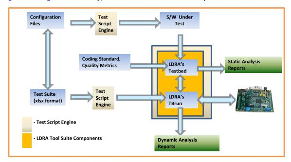
Figure 2. Automated Static and Dynamic Analysis Flow
