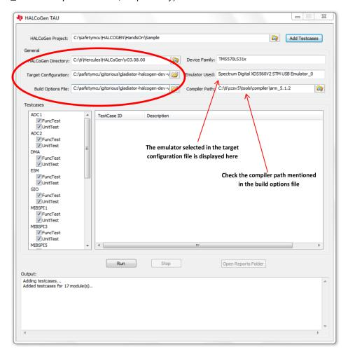
Figure 8. Target and Build Option Selection
