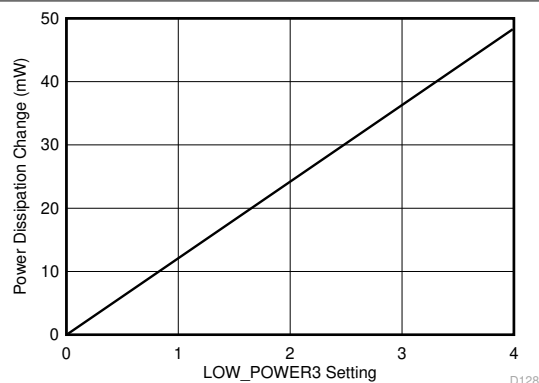
Figure 6-11. Power Dissipation Change vs LOW_POWER3 register setting
