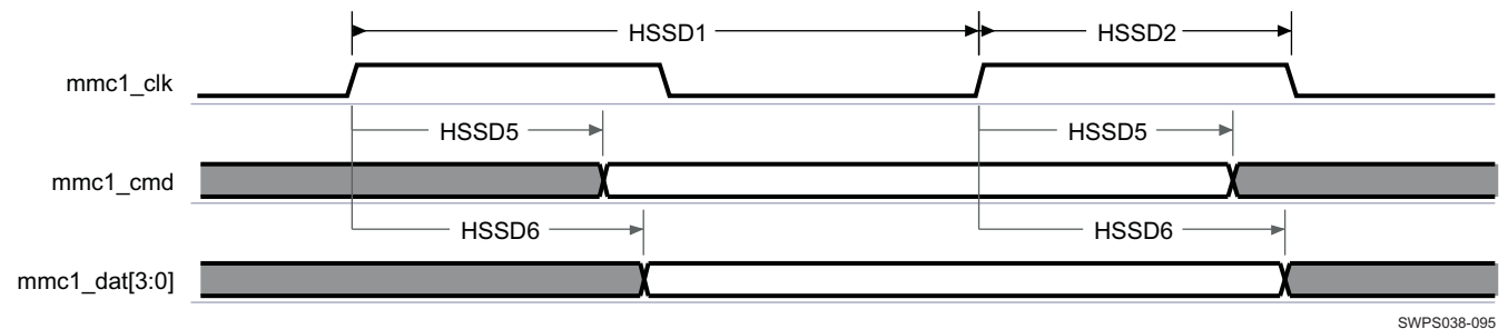
Figure 6-66. MMC1 Interface—High-Speed SD Mode—Data/Command Transmit
